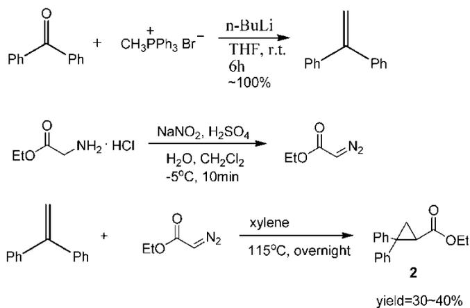
1,1-Diphenylethene was quantitatively prepared by Wittig reaction from benzophenone. Ethyl glycinate hydrochloride was diazotized to ethyl
