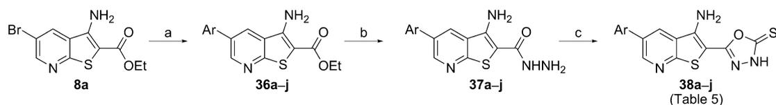
**Scheme 8.** Reagents and conditions: a) ArB(OH)<sub>2</sub>, K<sub>2</sub>CO<sub>3</sub>, Pd(PPh<sub>3</sub>)<sub>4</sub>, 1,4-dioxane, H<sub>2</sub>O; b) hydrazine hydrate, EtOH, reflux; c) CS<sub>2</sub>, pyridine, reflux.
