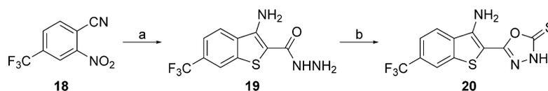
**Scheme 3.** Reagents and conditions: a) thioacetic acid hydrazide, *t*BuOK, DMF, 0 °C; b)  $\text{CS}_2$ , pyridine, 90 °C.
