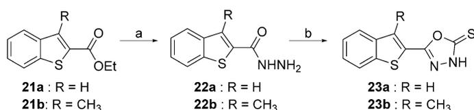
**Scheme 4.** Reagents and conditions: a) hydrazine monohydrate, EtOH, reflux; b) CS<sub>2</sub>, pyridine, 90 °C.
