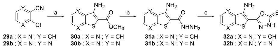
**Scheme 6.** Reagents and conditions: a) methyl thioacetate, Et<sub>3</sub>N, MeOH, reflux; b) hydrazine hydrate, EtOH, reflux; c) CS<sub>2</sub>, pyridine, reflux.
