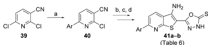
**Scheme 9.** Reagents and conditions: a) ArB(OH)<sub>2</sub>, K<sub>2</sub>CO<sub>3</sub>, Pd(PPh<sub>3</sub>)<sub>4</sub>, 1,4-dioxane, H<sub>2</sub>O; b) ethyl 2-thioacetate, K<sub>2</sub>CO<sub>3</sub>, EtOH, reflux; c) hydrazine hydrate, EtOH, reflux; d) CS<sub>2</sub>, pyridine, reflux.
