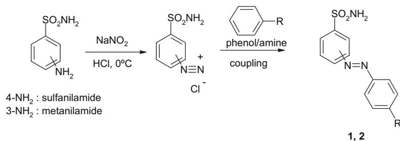
**Scheme 1.** Preparation of diazenylbenzenesulfonamides **1** and **2** by diazotization of sulfanilamide/metanilamide followed by coupling with phenols/amines.
