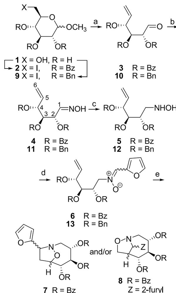
Figure 3. a: (**2**→**3**, **9**→**10**): Zn, sonication (1.6 g scale: 90%, 5 g scale: 30%) or Zn and Co(II)phthalocyanine (5 g scale: 70%), b:  $NH_2OH \cdot HCl$ ,  $NaHCO_3$  (70%), c:  $NaBH_3CN$ ,  $HCl/dioxane$ , d: 2-furaldehyde, toluene (c + d: 30–40%),  $4 \text{ \AA}$  MS,  $50^\circ C$ , 18 h, e: toluene,  $120^\circ C$ ,  $4 \text{ \AA}$  MS, Lewis acid catalyst, **7**: 9-oxa-1-azabicyclo-[4.2.1]nonane, **8**: 8-oxa-1-azabicyclo-[4.2.1]nonane skeletons.
