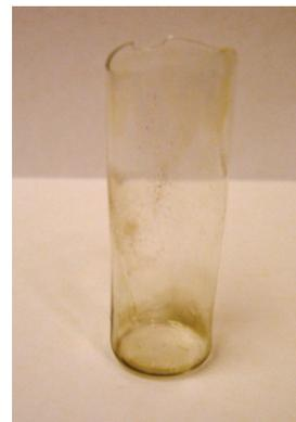
FIGURE 3. A thimble after the oxidation of styrene in DMF/H<sub>2</sub>O, partitioning of the product to the exterior with 25 mL of hexanes, and decanting of solvent from the interior. The thimble is mostly clear, which reflects the presence of very little Pd on the interior of the PDMS matrix.
