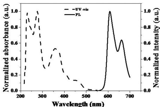
**Figure 1.** Absorption of UV-vis (left axis) and PL (right axis) spectra of the Ir-DMBQ(NBT)<sub>2</sub> complex **B** in dichloromethane ( $1.0 \times 10^{-6}$  mol/L).
