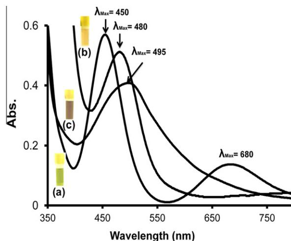
Fig. 2. UV–Vis spectra of (a) green  $RuCl_2(dppb)_2(\mu-dppb)$ , (b) yellow **1**, (c) brown **2** complexes direct dissolved in  $CHCl_3$  at RT. (For interpretation of the references to colour in this figure legend, the reader is referred to the web version of this article.)
