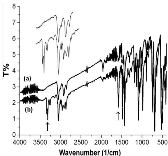
Fig. 1. IR-KBr disk spectra of (a)  $RuCl_2(dppb)_2(\mu-dppb)$  and (b) complex **1**.
