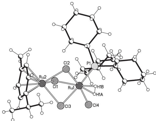
**Figure 4.** Graphic representation of the molecular structure of complex **8** in the crystal. The solvent molecules (1.5 toluene) are not shown for clarity. Selected bond lengths (Å) and angles (deg): Ru1–Cl1 2.4532(16), Ru1–Cl2 2.4194(19), Ru1–Cl3 2.5468(18), Ru1–Cl4 2.3902(19), Ru1–P1 2.2871(19), Ru1–H1A 1.67(7), Ru1–H1B 1.79(7), Ru1···Ru2 3.2747(9); P1–Ru1–Cl1 98.84(6), P1–Ru1–Cl4 91.68(7), P1–Ru1–Cl2 96.55(6), Cl4–Ru1–Cl2 170.66(6).
