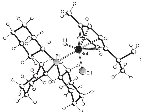
**Figure 1.** Graphic representation of the molecular structure of complex **3** in the crystal. Selected bond lengths (Å) and angles (deg): Ru1–Cl1 2.4393(12), Ru1–H1 1.48(5), Ru1–P1 2.3222(12); P1–Ru1–Cl1 89.64(4), P1–Ru1–H1 75.8(18), Cl1–Ru1–H1 88.9(17).
