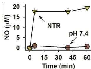
**Figure 3.** Nitric oxide released during decomposition of **4b** (50  $\mu\text{M}$ ) in the presence of NTR in pH 7.4 phosphate buffered saline.
