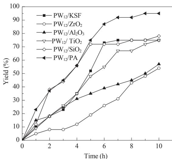
Fig. 3. Effect of the different supported- $PW_{12}$  compounds in the reaction of chalcone with phenylhydrazine. Reaction conditions: chalcone 1 mmol, phenylhydrazine 1 mmol, and supported- $PW_{12}$  (2 mol%) in solvent (5 ml) after 10 h at  $45\text{ }^{\circ}\text{C}$ .
