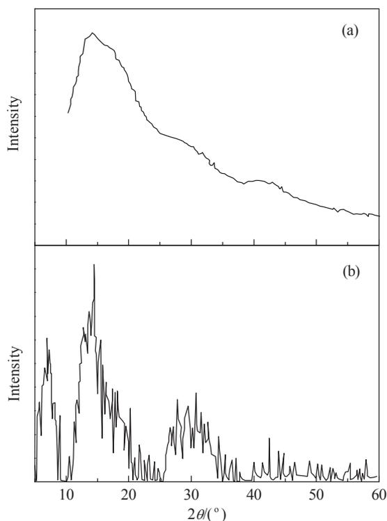
Fig. 1. XRD patterns of PA (a) and PW<sub>12</sub>/PA (b).
