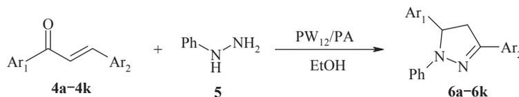
Scheme 2. Catalytic synthesis of 1,3,5-triaryl-2-pyrazoline derivatives (**6**) from chalcone and phenylhydrazine over  $\text{PW}_{12}/\text{PA}$ .
