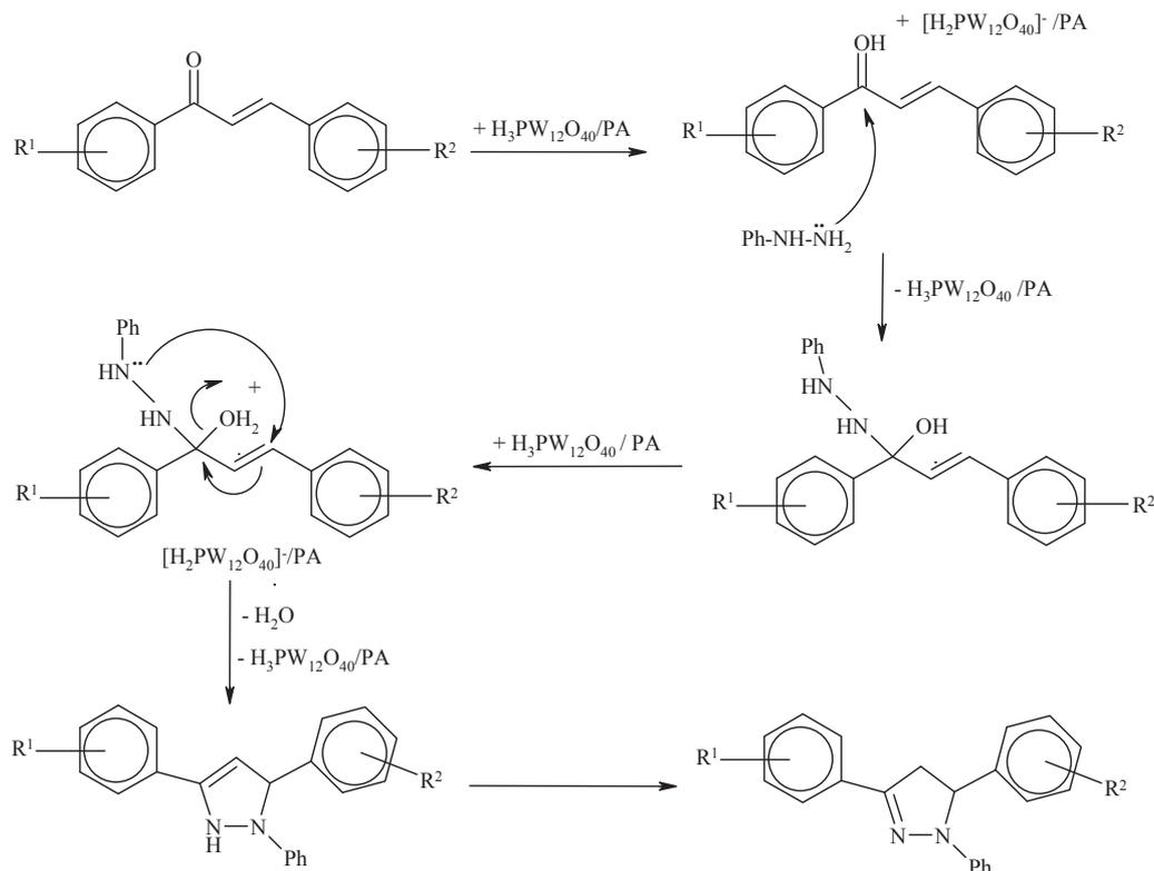
**Scheme 3.** Suggested mechanism for the reaction of chalcone with phenylhydrazine in the presence of  $\text{PW}_{12}/\text{PA}$ .
