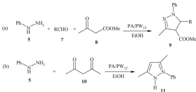
**Scheme 4.** Preparation of other types of 2-pyrazolines in the presence of  $\text{PW}_{12}/\text{PA}$ .
