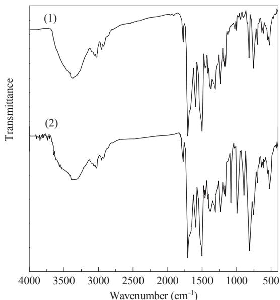
Fig. 2. FT-IR spectra of PA (1) and  $PW_{12}/PA$  (2).
