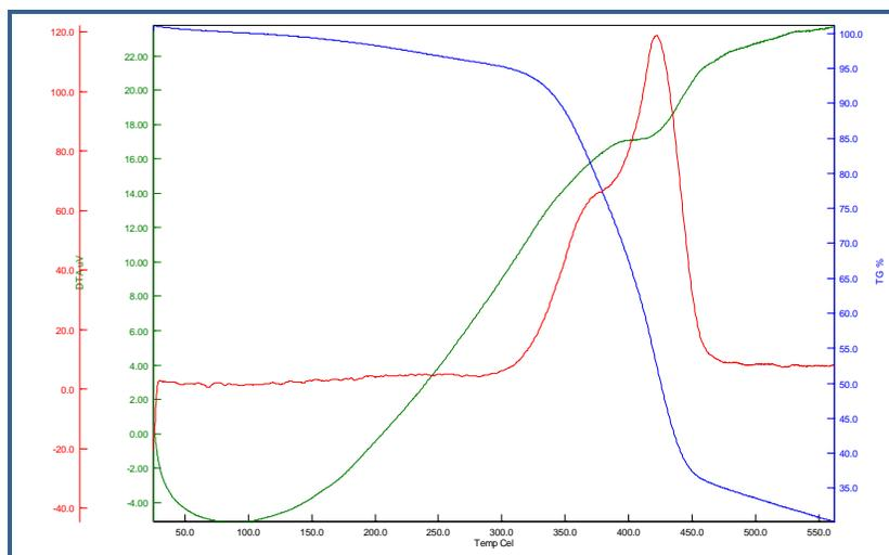
**Figure 6** TG-DTA patterns of BBC-Polym@BBY@Pd in N<sub>2</sub> atmosphere
