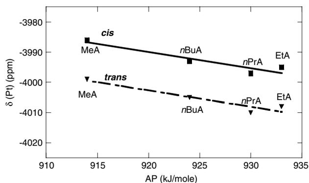
Fig. 2.  $\delta(\text{Pt})$  of the linear aliphatic amine dimers vs. proton affinity of the amine [19–21].
