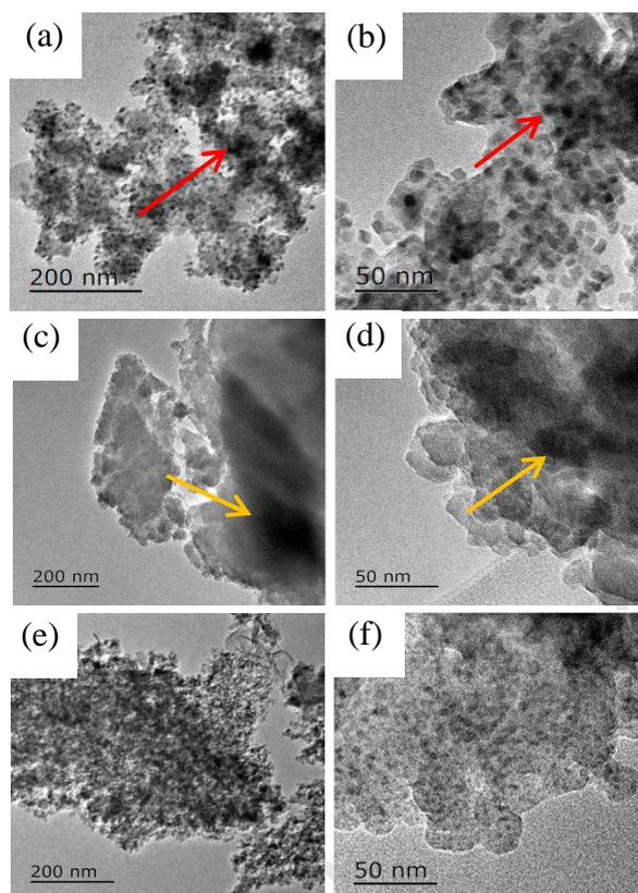
Fig. 4. TEM photographs of the catalysts: (a), (b) S-20; (c), (d) C-20; (e), (f) I-20.
