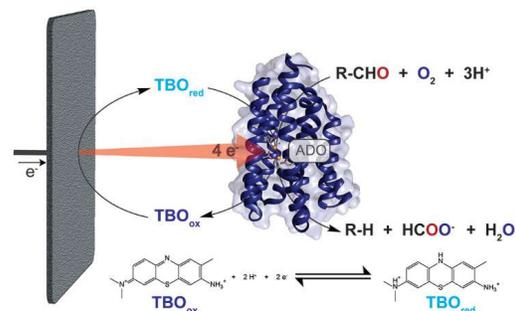
**Scheme 2.** Schematic of the PmADO biocathode.
