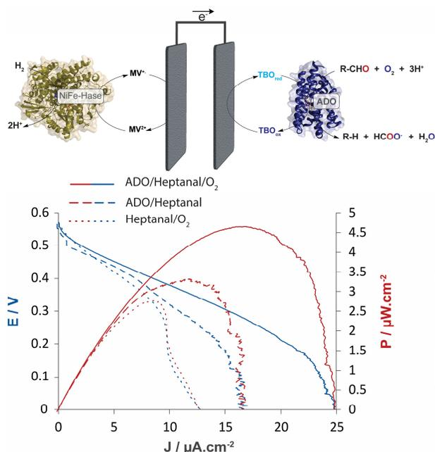
**Figure 3:** Representative power (red lines) and polarization curves (blue lines) for  $\text{H}_2$ /heptanal fuel cells (solid lines); a control fuel cell without ADO in the presence of  $\text{O}_2$  and heptanal (dotted lines), and a control with ADO in the presence of heptanal without  $\text{O}_2$  (dashed lines). The measurements were performed by linear sweep polarization at  $0.2 \text{ mV s}^{-1}$  with vigorous stirring.
