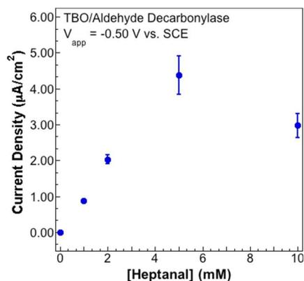
**Figure 2.** Heptanal-induced changes in the catalytic reduction current by TBO-mediated PmADO with a  $-0.5\text{ V}$  applied potential.
