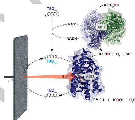
**Scheme 3:** Illustration of the bioelectrochemical system combining PmADO and ADH.
