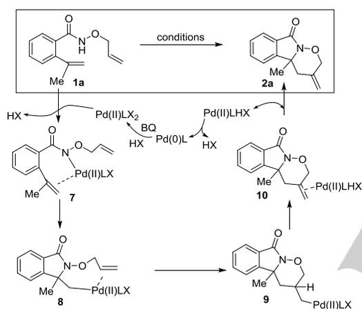
Scheme 7. Proposed Catalytic Cycle.
