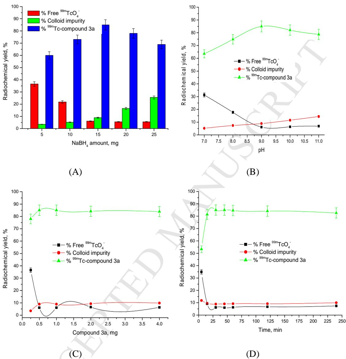
**Fig. 2.** Factors affecting radiochemical yield of  $^{99m}\text{Tc}$ -compound 3a complex.
