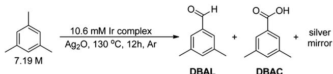
and mesitylene as solvent in excess, 3,5-dimethylbenzaldehyde (DBAL) and 3,5-dimethylbenzoic acid (DBAC) were produced (2.9 turnovers total; entry 1 in Table 3). Silver mirror deposited on the glass wall of the reaction vessel, consistent with reduction of  $Ag_2O$  to  $Ag(0)$ . The result was reproducible (entry 2).
