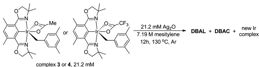
**Oxidation of (Phebox)Ir Complexes 1, 2, 3, and 4 by One Equivalent of Ag<sub>2</sub>O.** We considered the question of whether the catalytic oxidation of mesitylene proceeded via C–H activation followed by oxy-functionalization<sup>59,79</sup> or via Ir-oxo formation followed by C–H hydroxylation.<sup>52,59</sup> DFT calculations suggested that both pathways (Figure 2) could be energetically accessible.
