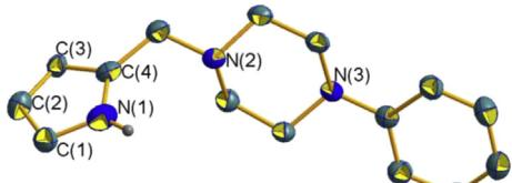
**Fig. 1.** The molecular structure of compound **1**. The thermal ellipsoids were drawn at 30% probability. All of the hydrogen atoms except the one on the pyrrole nitrogen atom were omitted for clarity.
