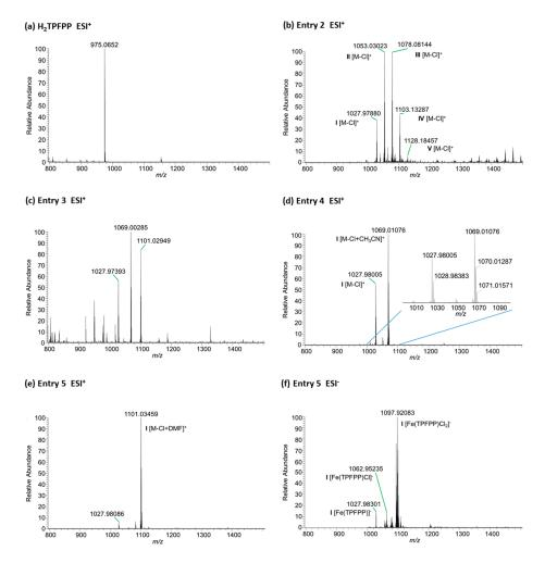
**Figure 3.** High Resolution ESI mass spectra analysis of  $H_2$ TPFPP (**a**) and of iron complexes obtained under the experimental conditions described in Table 1, Entry 2 (**b**); Entry 3 (**c**); Entry 4 (**d**); Entry 5 (**e**,**f**).
