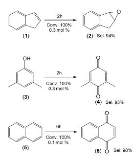
Figure 5. Catalytic oxidation of aromatic compounds in the system [Fe(TPFPP)Cl]/EtOH/H<sub>2</sub>O<sub>2</sub>.
