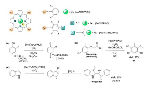
**Figure 1.** Oxidations of aromatic compounds in the presence of Mn(III) or Fe(III)porphyrins: (a) oxidation of alkylphenols; (b) oxidation of the herbicide mecoprop; (c) production of indigo dye from indene oxidation.
