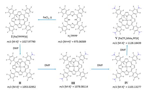
**Figure 4.** Complexes of [Fe(TPFPP)X] obtained during metalation reactions by heating DMF and pyridine mixtures for long reaction periods.
