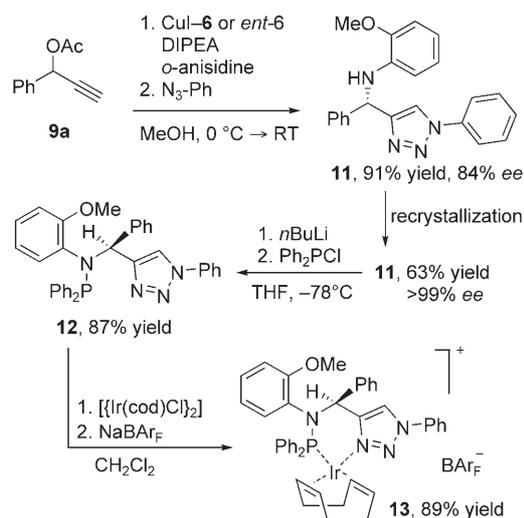
**Scheme 3.** Synthesis of the chiral ClickPhine ligand **12** and the Ir<sup>I</sup> complex **13**. cod = 1,5-cyclooctadiene, BAR<sub>F</sub> = tetrakis[3,5-bis(trifluoromethyl)phenyl]borate.
