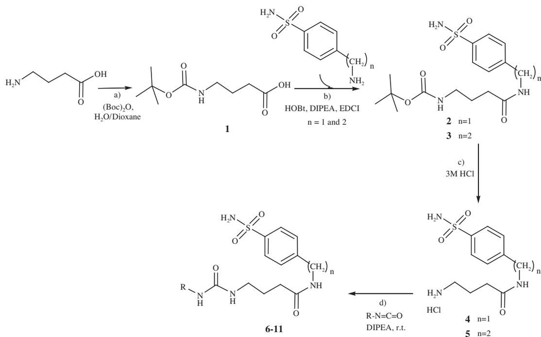
**Scheme 1.** Preparation of sulfonamides **6–11** by reaction of 4-amino-*N*-(4-sulfamoyl-benzyl)-butyramide hydrochloride ( $n = 1$ ) (**4**) or 4-amino-*N*-[2-(4-sulfamoyl-phenyl)-ethyl]-butyramide hydrochloride ( $n = 2$ ) (**5**) with isocyanates (R–NCO) in presence of diisopropylethylamine (DIPEA), in acetonitrile (dry).
