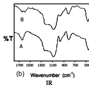
**Figure 2.** (a) XRD pattern and (b) infrared spectra. A: MCM-48/H<sub>5</sub>PW<sub>10</sub>V<sub>2</sub>O<sub>40</sub> before reaction; B: MCM-48/H<sub>5</sub>PW<sub>10</sub>V<sub>2</sub>O<sub>40</sub> after recycling.
