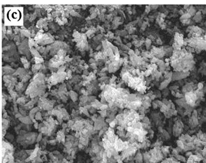
**Figure 1.** (a) Low-angle XRD patterns of calcined MCM-48 and MCM-48/H<sub>5</sub>PW<sub>10</sub>V<sub>2</sub>O<sub>40</sub>. SEM images of (b) MCM-48 and (c) MCM-48/H<sub>5</sub>PW<sub>10</sub>V<sub>2</sub>O<sub>40</sub>.
