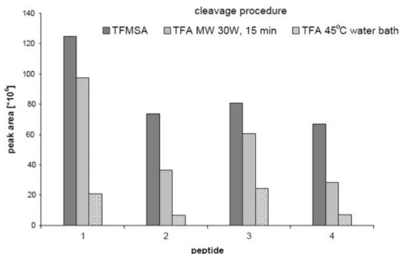
**Figure 2.** The comparison of HPLC peak areas of peptides 1–4 cleaved from the Merrifield resin using standard TFMSA procedure, TFA with microwave irradiation (30 W, 15  $\times$  1 min) and TFA at elevated temperature 45 °C (water bath). Fifty-milligram resin samples from the same synthetic batch were used in each case.
