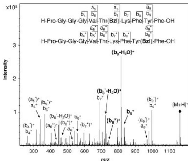
**Figure 7.** The MS/MS spectrum of the ion  $m/z = 1162.6$ , corresponding to peptide 5 with one protective benzyl group preserved (FT-ICR, collision energy of 30 eV). The asterisks indicate the daughter ion series produced when the benzyl group is located on Tyr residue.
