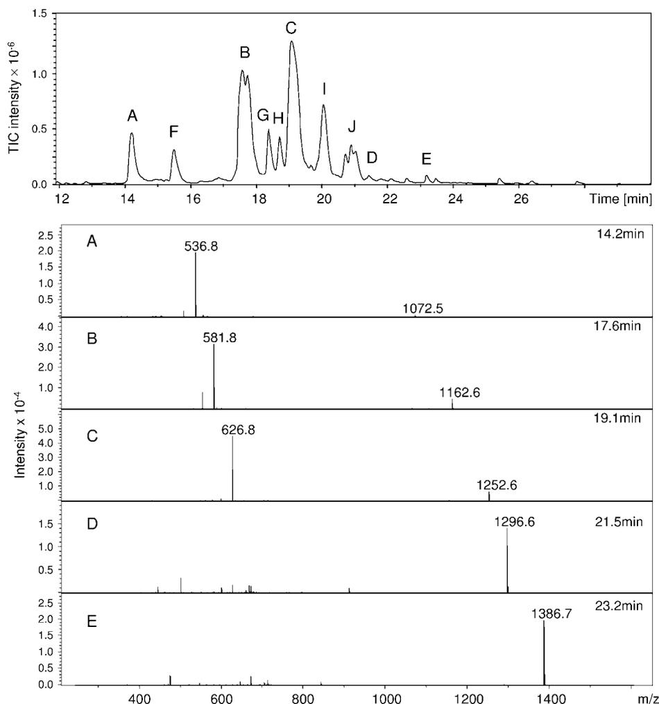
**Figure 5.** Top panel: the LC–MS chromatogram of crude peptide 5 obtained after 15-min MW-assisted TFA cleavage from Merrifield resin (total ion current, positive ion mode). Chromatographic peaks A–E correspond to forms of peptide 5 with various protection level, peaks F–J represent methylated forms of compounds A–E. Panels A–E: mass spectra of peaks of deprotected (A) and partially protected (B–E) forms of peptide 5.
