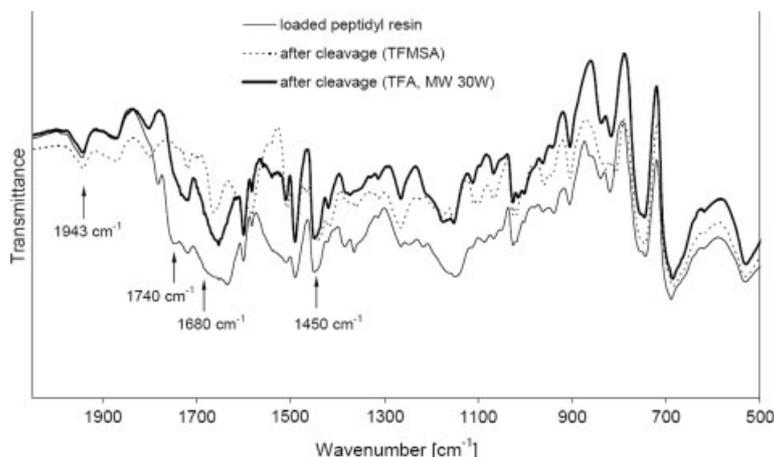
**Figure 4.** The comparison of IR spectra: resin loaded with the peptide 1 (thin line), the resin after TFMSA deprotection (dotted line) and TFA–MW deprotection (thick line).
