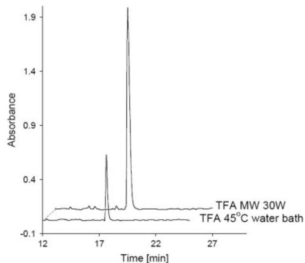
**Figure 3.** The HPLC profiles of peptide 4 removed from the Merrifield resin using TFA in water bath at elevated temperature and in MW reactor.
