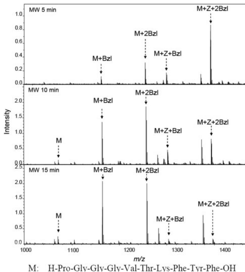
**Figure 6.** The mass spectra of peptide 5 after MW-assisted TFA cleavage from Merrifield resin after 5, 10 and 15 min of irradiation (negative ion mode).
