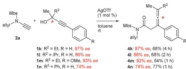
**Scheme 2** Central-to-axial chirality transfer from optically active **1k–1n** to optically active **4k–4n**.
