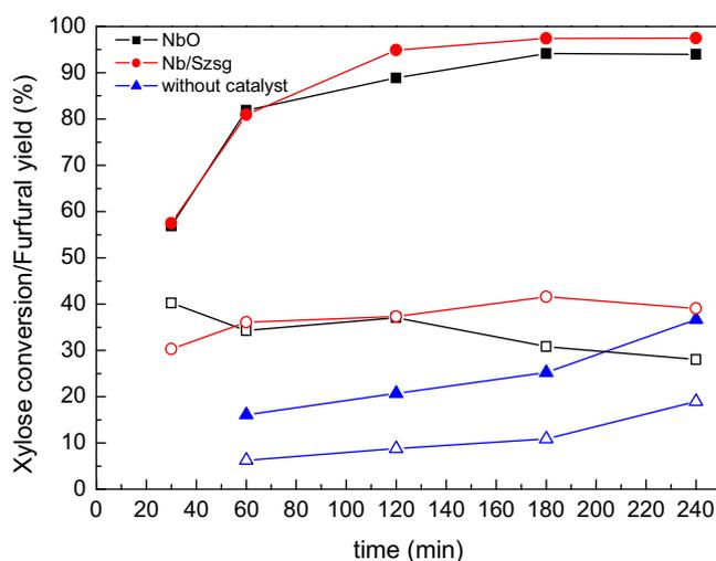
**Fig. 7.** Comparison of the xylose conversion (filled markers) and furfural yield (empty markers) for NBO and Nb/SZ<sub>sg</sub> catalysts and without catalyst (blank test) vs. reaction time. Reaction conditions: 10 wt.% of xylose and 5 wt.% of catalyst in the aqueous phase, CPME/aqueous phase mass ratio, 2.33; 50 g total solution; reaction temperature, 180 °C.
