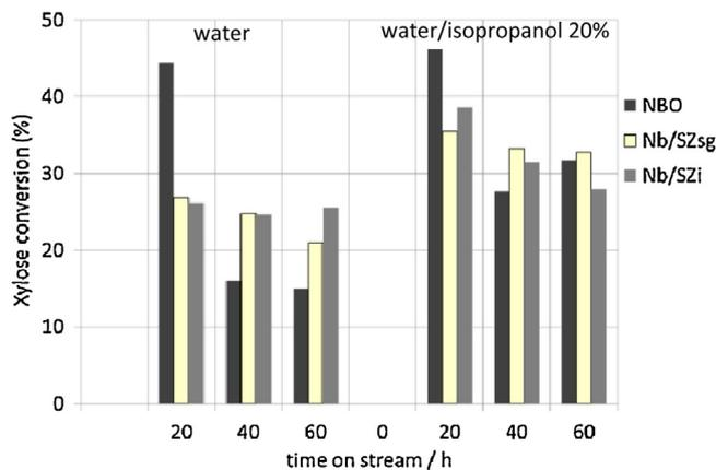
**Fig. 5.** Xylose conversion for different time on stream for the NBO and Nb/SZ catalysts. Reaction conditions: fixed bed reactor; 4.5 wt.% xylose, 3 wt.% catalyst; contact time, 6–10 min  $\text{g mL}^{-1}$ ; reaction temperature, 130 °C.
