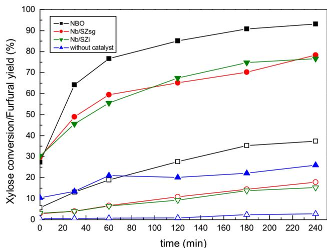
**Fig. 6.** Comparison of the xylose conversion (filled markers) and furfural yield (empty markers) with reaction time on NBO and Nb/SZ catalysts and without catalyst (blank test). Reaction conditions: batch reactor; 2 wt.% xylose and 0.2 wt.% of catalyst;  $\gamma$ -valerolactone/aqueous mass ratio, 9; 50 g total solution; reaction temperature, 160 °C.
