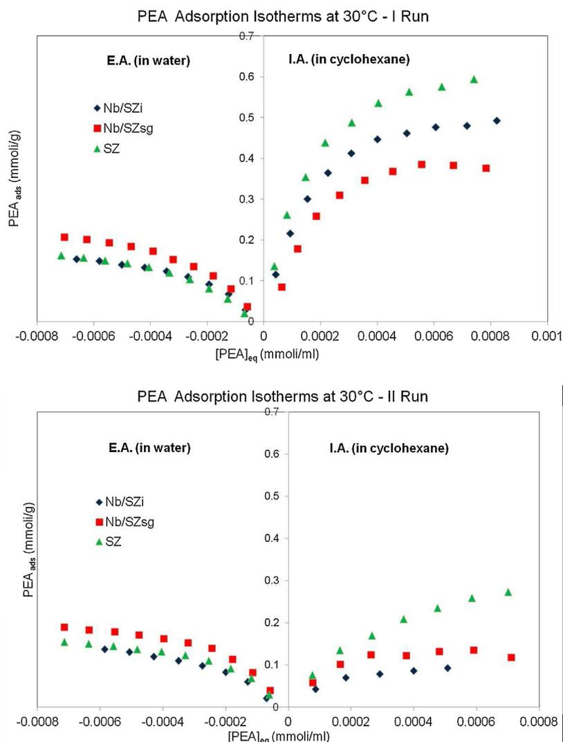
**Fig. 3.** Intrinsic (in cyclohexane) and effective (in water) acidities of the samples: adsorption isotherms of PEA at 30 °C. I° run collected on fresh and activated sample and II° run collected on the previously sample saturated by PEA and eluted with solvent.
