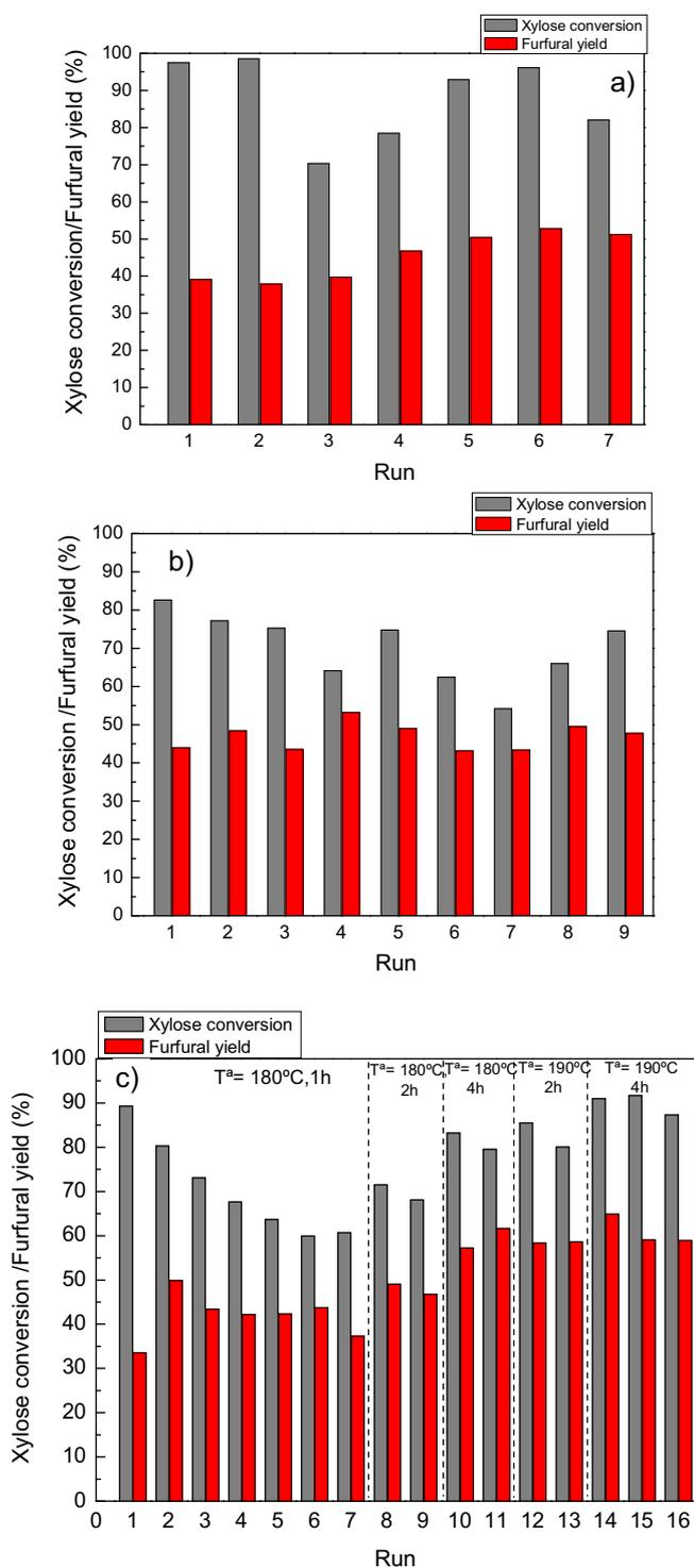
**Fig. 8.** Recycling tests on NBO and Nb/SZ catalysts: a) Nb/SZ<sub>sol</sub>, b) Nb/SZ<sub>i</sub>, c) NBO. Reaction conditions: 10 wt.% xylose and 5 wt.% catalyst in the aqueous phase, CPME/aqueous phase mass ratio, 2.33; 50 g total solution, reaction temperature, 180 °C, time of reaction, 240 min for the supported catalysts.
