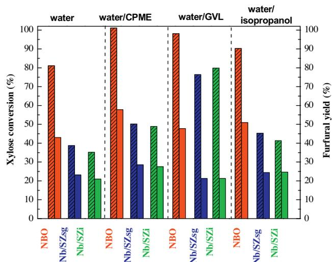
**Fig. 4.** Xylose conversion (dashed bars) and furfural yield (filled bars) for the NBO and Nb/SZ catalysts in different reaction solvents. Reaction conditions: batch reactor; 4.5 wt.% xylose, 3 wt.% catalyst; 5 g total solution;  $\gamma$ -valerolactone (GVL)/aqueous mass ratio, 9; CPME/aqueous mass ratio, 2.33; water/isopropanol 20% v/v; reaction temperature, 130 °C; tos, 360 min.
