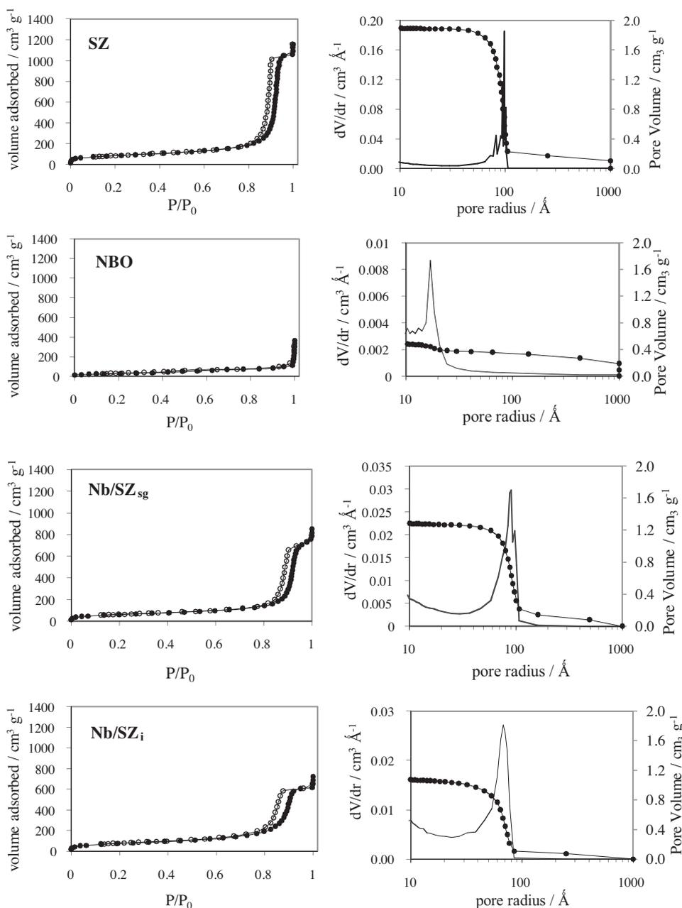
Fig. 2.  $N_2$  adsorption/desorption isotherms (left side) and BJH pore volume distribution (right side) of all the catalyst samples.
