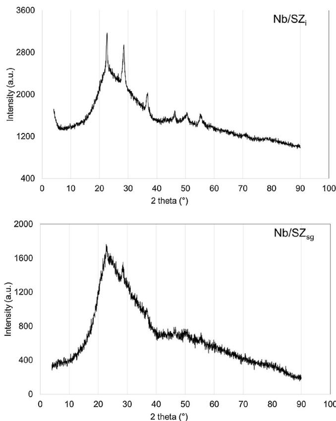
Fig. 1. P-XRD of Nb/SZ<sub>i</sub> (top) and Nb/SZ<sub>sg</sub> (bottom) (P-XRD of NBO is shown in Supporting Information section, Figure 3S).
