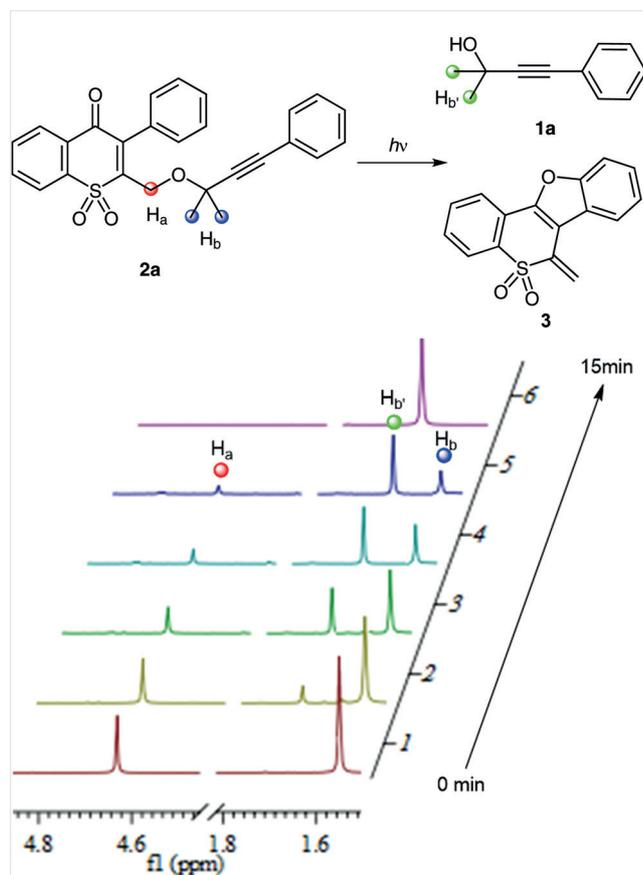
**Figure 2** Sections of the  $^1\text{H}$  NMR spectrum ( $\delta = 1.5\text{--}4.8$  ppm) of a 0.01 M solution of **2a** in  $\text{CDCl}_3$  recorded after 0, 3, 6, 9, 12, and 15 min of irradiation.
