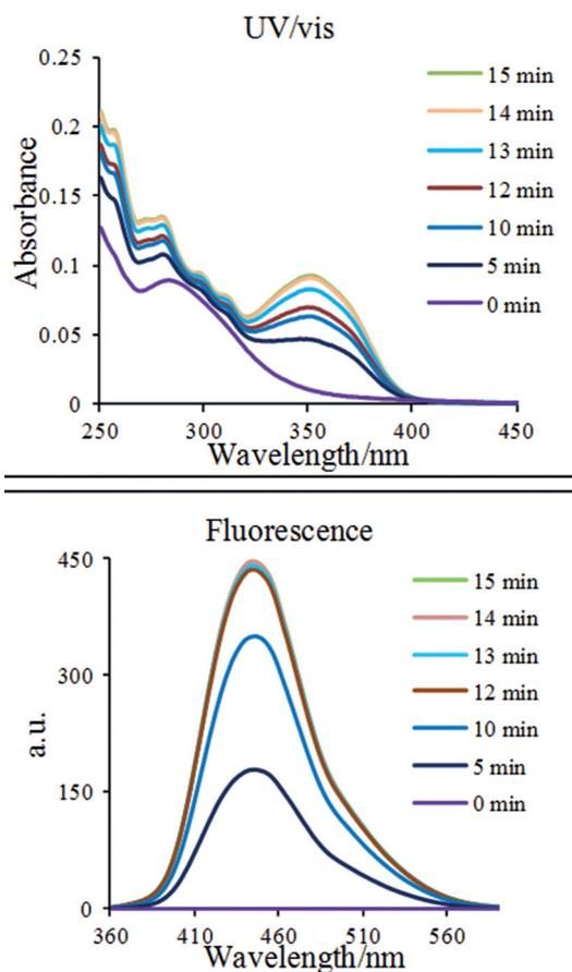
**Figure 4** UV-vis and fluorescence spectra upon excitation at 350 nm of a  $1.0 \times 10^{-5}$  M methanolic solution of **2a**, recorded after 0, 5, 10, 12, 13, 14, and 15 min of irradiation
