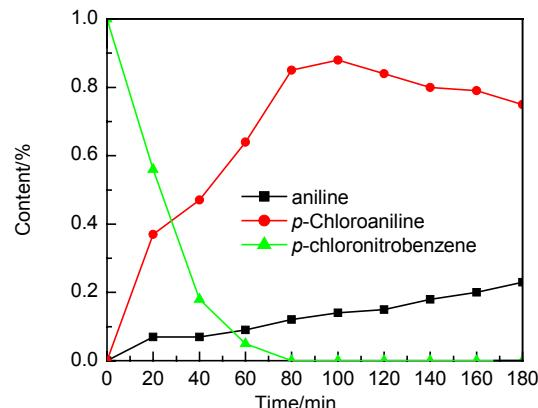
**Figure 3** Pd/C catalyzed hydrogenation of *p*-chloronitrobenzene with N<sub>2</sub>H<sub>4</sub>•H<sub>2</sub>O. Reaction conditions: *p*-chloronitrobenzene, 1.0 mmol; Pd/C catalyst (Pd: 5.0 wt%), 16 mg; N<sub>2</sub>H<sub>4</sub>•H<sub>2</sub>O, 3.0 mmol; at 25 °C; 2.0 mL toluene as solvent.
