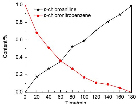
**Figure 2** MoS<sub>2</sub> catalyzed hydrogenation of *p*-chloronitrobenzene with N<sub>2</sub>H<sub>4</sub>•H<sub>2</sub>O. Reaction conditions: *p*-chloronitrobenzene, 1.0 mmol; MoS<sub>2</sub> catalyst, 16 mg; N<sub>2</sub>H<sub>4</sub>•H<sub>2</sub>O, 3.0 mmol; at 25 °C; 2.0 mL toluene as solvent.
