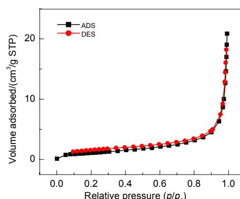
**Figure 1** Nitrogen adsorption-desorption isotherms of MoS<sub>2</sub>.
