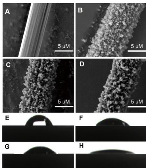
**Figure 1.** Scanning electron microscopy (SEM) images of (A) bare CFE, (B) PEDOT/CFE, (C) PEDOT-OH/CFE, and (D) PEDOT-PC/CFE. The contact angles of (E) GC, (F) PEDOT/GC, (G) PEDOT-OH/GC and (H) PEDOT-PC/GC.
