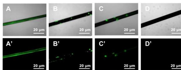
**Figure 2.** Confocal fluorescent images of FITC-BSA treated electrodes. (A, A') bare CFE, (B, B') PEDOT/CFE, (C, C') PEDOT-OH/CFE, (D, D') PEDOT-PC/CFE in merged (upper) and dark (lower) fields.
