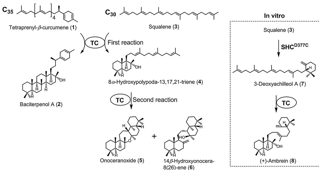
**Scheme 1.** Cyclization of **1** and **3** catalyzed by TC, and enzymatic synthesis of **8** by using SHC<sup>D377C</sup> and TC.
