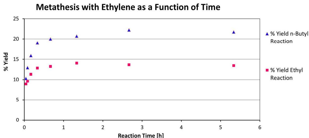
**Figure 4.** Results of the time-dependent cross-metathesis between ethyl or *n*-butyl crotonate and ethylene catalyzed by the Hoveyda-Blechert catalyst (reaction conditions as denoted in Scheme 6). Each data point is the end point of an experiment which was stopped at the indicated time.
