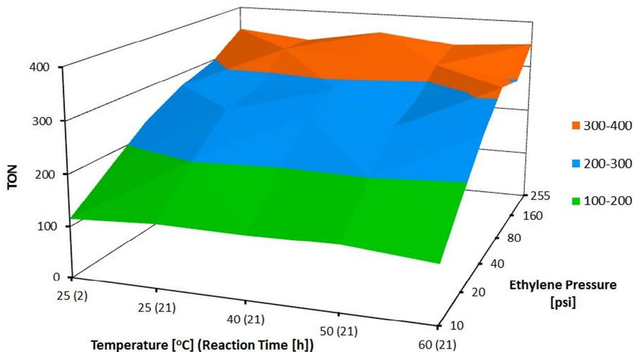
**Figure 3.** Contour map of the experimental results of the temperature- and pressure-dependent cross-metathesis between ethyl crotonate and ethylene using the Hoveyda-Blechert catalyst (reaction conditions as denoted in Scheme 4).
