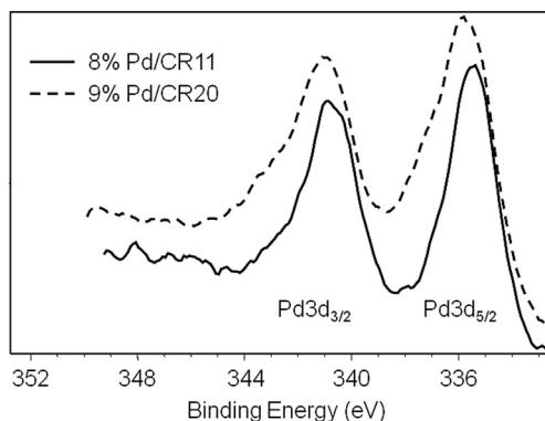
**Fig. 3.** XPS spectra of 8% Pd/CR11 and 9% Pd/CR20.
