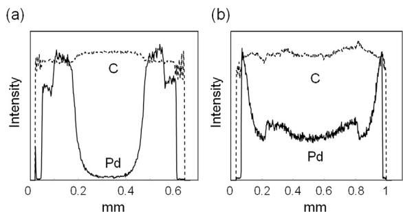
**Fig. 2.** (a) EPMA of 8% Pd/CR11 and (b) 9% Pd/CR20.
