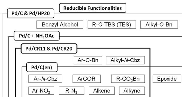
**Fig. 4.** Chemoselectivity of 8% Pd/CR11- and 9% Pd/CR20-catalyzed hydrogenations.
