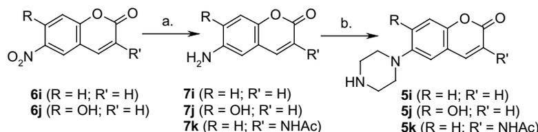
**Scheme 3.** Reagents and conditions: (a) Raney-Ni, H<sub>2</sub>, MeOH; (b) bis-(2-chloro ethyl)-ammonium chloride, NMP.
