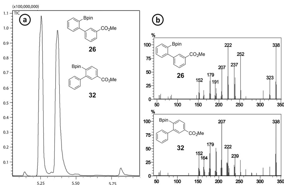
Figure 4. (a) GC–MS trace from the reaction mixture of the borylation of **25** displaying both regioisomers (**26** and **32**), which were formed in a 1:1 ratio. (b) Mass-spectrometric analysis of both GC signals. Both regioisomers give closely related patterns because of their structural similarity.
