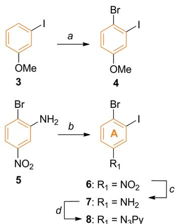
Scheme 1. Reagents and conditions: (a) NBS, MeCN, r.t., 15 h, 96%; (b) BF<sub>3</sub>·OEt<sub>2</sub>, ONO<sub>t</sub>Bu, THF, –30 °C to r.t., 3 h, then I<sub>2</sub>, KI, MeCN, r.t., 30 min, 97%; (c) Fe, HCl, EtOH, 0 °C, 2 h, 94%; (d) BF<sub>3</sub>·OEt<sub>2</sub>, ONO<sub>t</sub>Bu, CH<sub>2</sub>Cl<sub>2</sub>, –30 °C to r.t., 15 min, then pyrrolidine, K<sub>2</sub>CO<sub>3</sub>, r.t., 15 min, 95%; N<sub>3</sub>Py = diazenylpyrrolidine.
