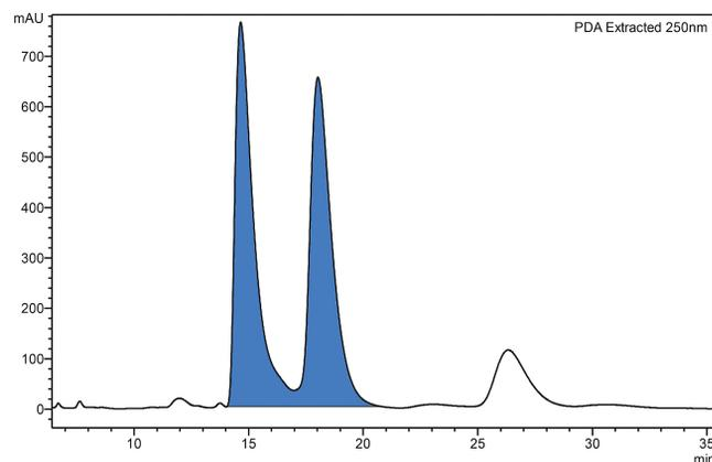
Figure 6. UV trace of a representative chiral HPLC run of the crude reaction mixture after filtration (Chiralpak IA; *n*-hexane/2-propanol (99:1), flow rate 1 mL/min, *T* = 25 °C). The chart reveals the two enantiomeric peaks (blue) as major compounds. The enantiomeric fractions were collected and combined to give 28% combined yield of the desired target structure **1**.
