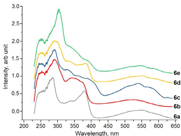
**Figure 5.** The UV absorption spectra of compounds **6a,b,c,d,e** in  $\text{CH}_2\text{Cl}_2$ .
