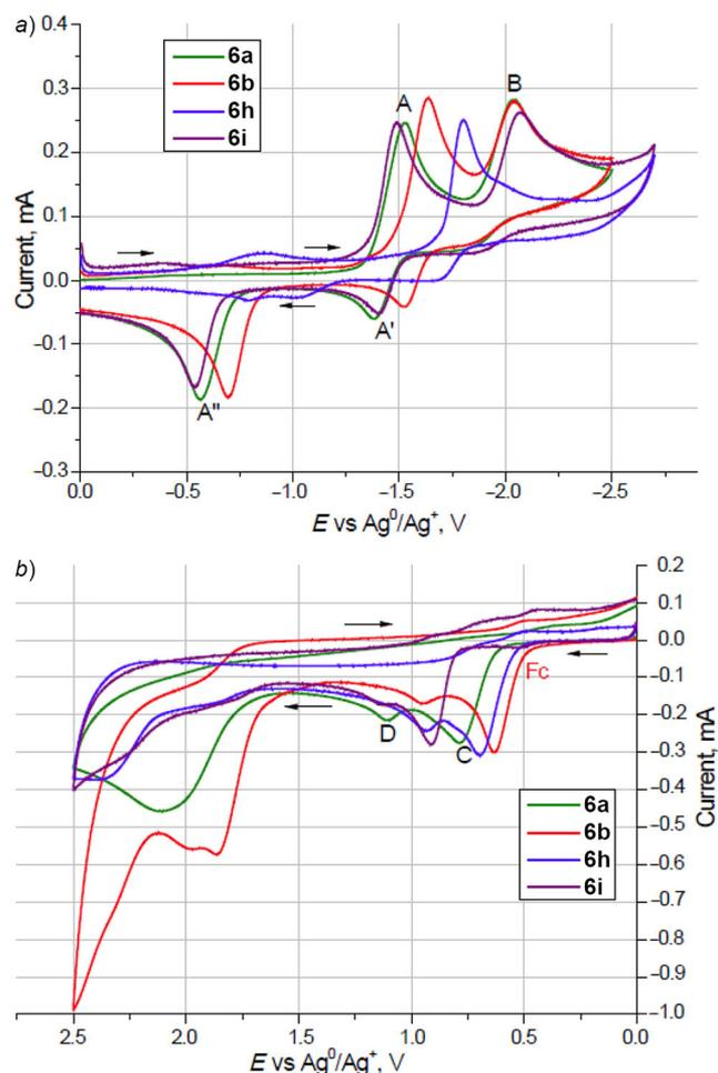
**Figure 8.** Cyclic voltammograms of compounds **6a,b,h,i** at a glassy carbon disk electrode with a) negative and b) positive scan directions; 1 mM solution in MeCN containing 0.1 M TBAP;  $\nu$  0.2 V/s.
