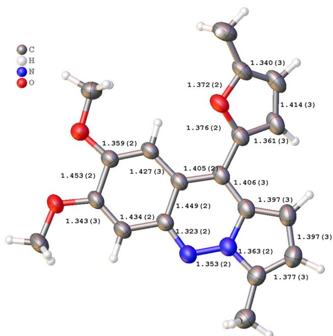
**Figure 1.** Molecular structure of compound **6b** with atoms represented as thermal vibration ellipsoids of 50% probability.
