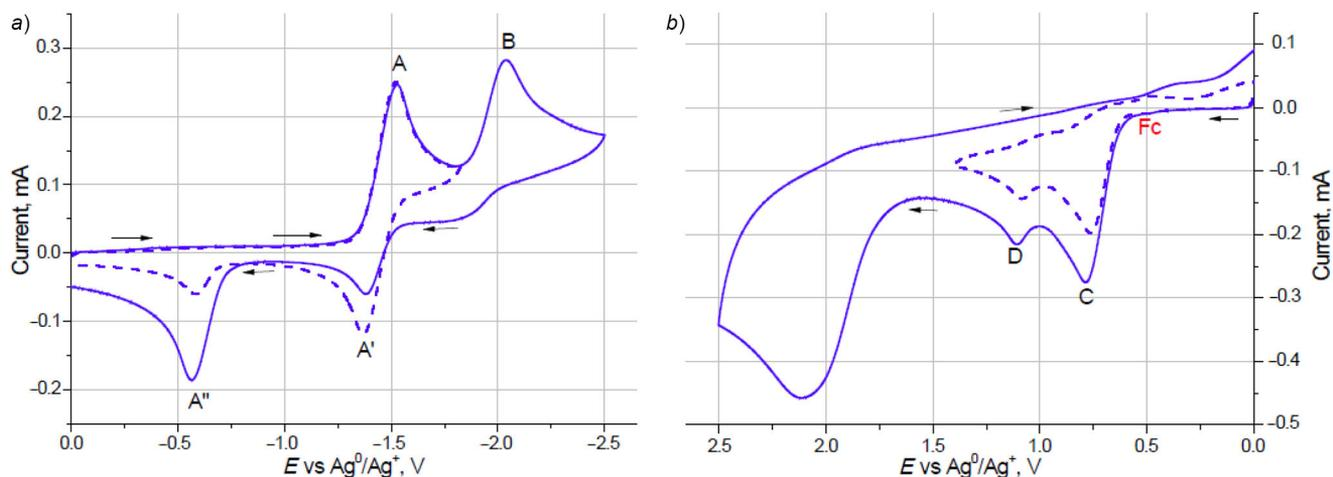
**Figure 6.** Cyclic voltammograms of compound **6a** at a glassy carbon disk electrode with a) negative and b) positive scan directions; 1 mM solution in MeCN containing 0.1 M TBAP;  $\nu$  0.2 V/s.
