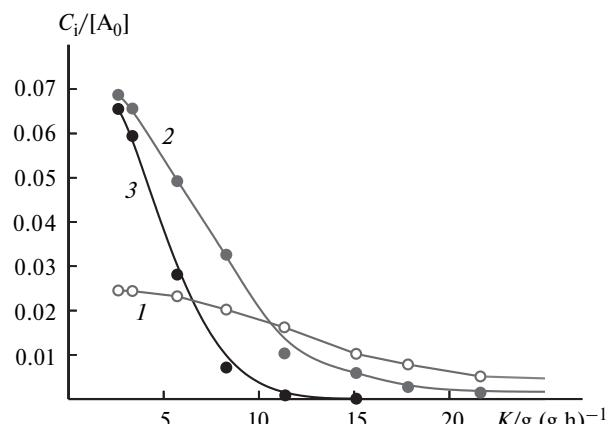
**Fig. 7.** Distribution of the dehalogenation products during hydrogenation of 3,4-DCNB in the presence of the 2.5%Pt/C catalyst under gradient-free flow conditions as a function of the contact load ( $K$ ): (1) PCA, (2) aniline, (3) 4-aminodiphenyl.
