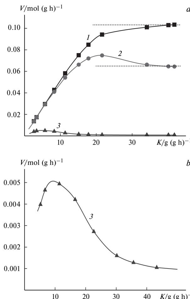
**Fig. 8.** Rates of 3,4-DCNB consumption (1), 3,4-DCA formation (2) and chloride-ion accumulation (3) vs. contact load during hydrogenation of 3,4-DCNB under gradient-free flow conditions (a). Initial region of the curve of chloride-ion accumulation (b).
