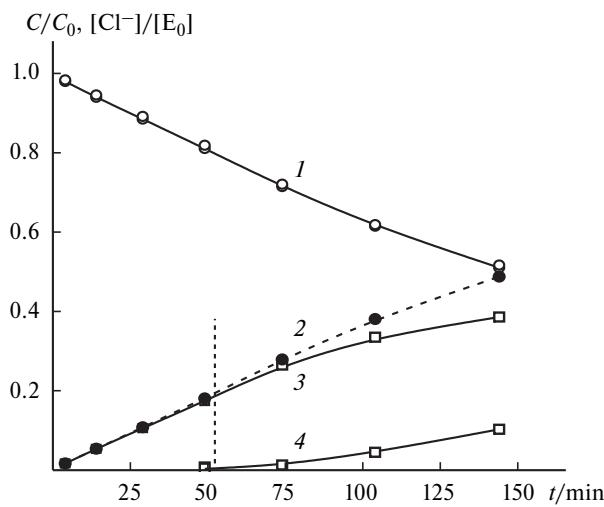
Fig. 3. Hydrogenation of PCA in 2-propanol at  $50 \pm 0.2^\circ\text{C}$  in the presence of the 2.5%Pt/C catalyst under static conditions: (1) consumption of PCA, (2) accumulation of chloride ions ( $[\text{Cl}^-]/[\text{E}_0]$ ,  $[\text{E}_0]$  is the initial PCA concentration), (3) formation of aniline, (4) formation of side products.
