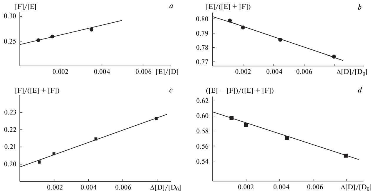
**Fig. 5.** Graphical analysis of Eqs (2)–(4) describing the initial segments of kinetic curves for dehalogenation of 3,4-DCA under static conditions: (*a*) Eq. (2), (*b*) Eq. (3), (*c*) Eq. 4, (*d*) difference between equations (3) and (4).
