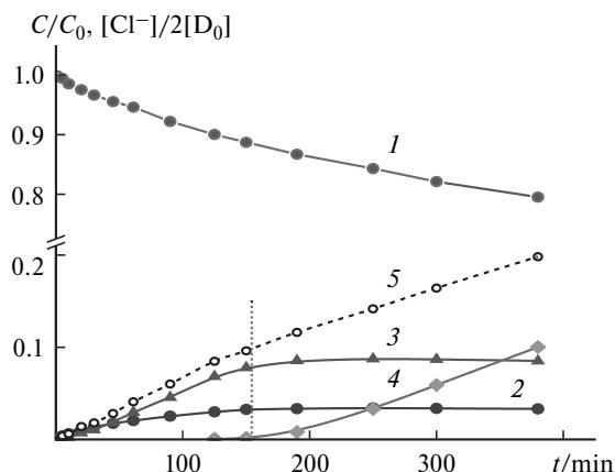
**Fig. 1.** Hydrogenation of 3,4-DCA in a solution of 2-propanol at  $50\pm0.2$  °C in the presence of the 2.5%Pt/C catalyst under static conditions: consumption of 3,4-DCA (1); formation of *p*-chloroaniline (2), aniline (3), and side products (4); accumulation of chloride ions ( $[\text{Cl}^-]/2[\text{D}_0]$ ) (5),  $[\text{D}_0]$  is the initial concentration of 3,4-DCA.
