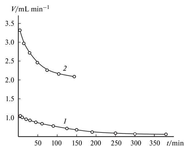
**Fig. 2.** Variation of the  $\text{H}_2$  absorption rate vs. time during hydrogenation of 3,4-DCA (1) and PCA (2) under static conditions.
