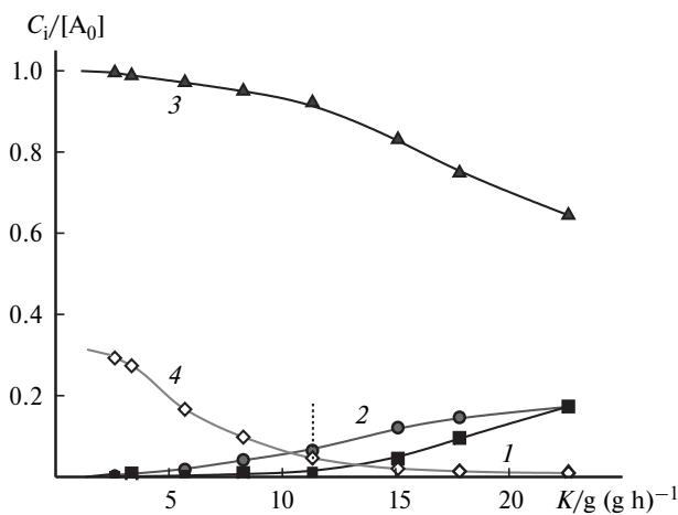
**Fig. 6.** Distribution of the relative concentrations ( $C_i/[A_0]$ ) of the products of 3,4-DCNB hydrogenation in the presence of the 2.5%Pt/C catalyst under gradient-free flow conditions as a function of contact load ( $K$ ): (1) 3,4-DCNB, (2) 3,4-DCPHA, (3) 3,4-DCA, (4) chloride ions. Here and in Figs 7 and 9,  $[A_0]$  is the initial concentration of 3,4-DCNB.
