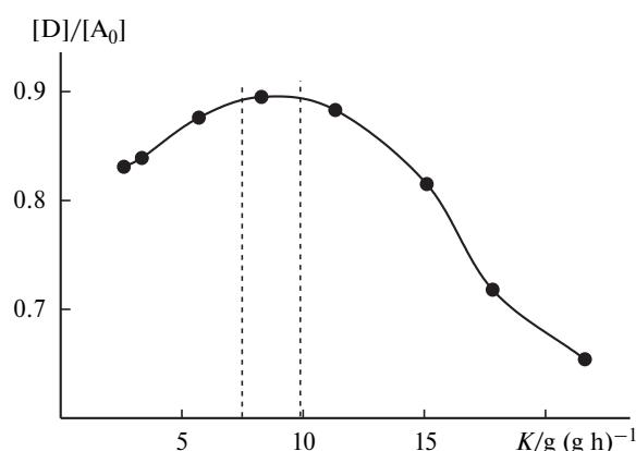
**Fig. 9.** Yield of 3,4-DCA vs. contact load during hydrogenation of 3,4-DCNB under gradient-free flow conditions.
