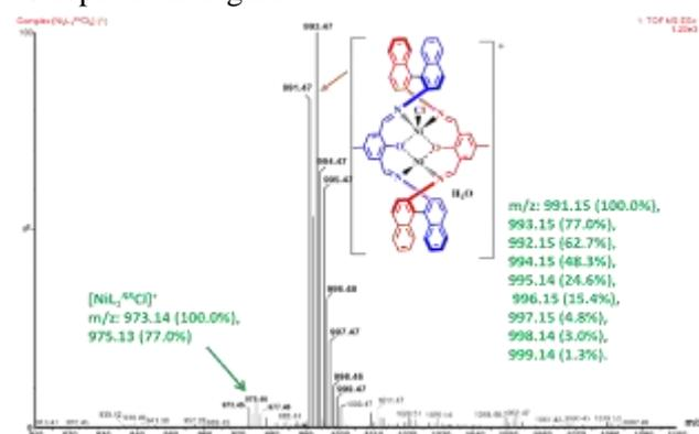
**Figure 1.** ESI-MS spectra of [Ni<sub>2</sub>L<sub>1</sub><sup>RR</sup>.Cl<sub>2</sub>] (**1**) helicate.
