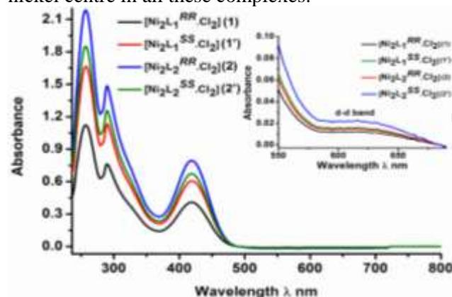
**Figure 2.** UV-Visible spectra of all the nickel helicates recorded in THF (1x10<sup>-5</sup>M). The inset shows d-d band (1x10<sup>-3</sup>M).
