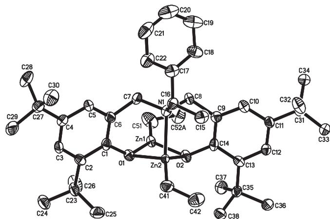
Fig. 1. X-ray structure of **3**. Hydrogen atoms, minor part of disordered atom C52 and the second independent molecule are omitted for clarity. Thermal ellipsoids are drawn at the 50% probability level.Table 1
