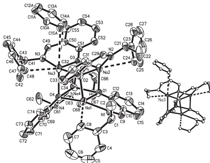
**Fig. 4.** X-ray structure of **7**. Hydrogen atoms are omitted for clarity. Thermal ellipsoids are drawn at the 50% probability level. Atoms C10a–C15a are generated by  $x - 1, y, z$ .
