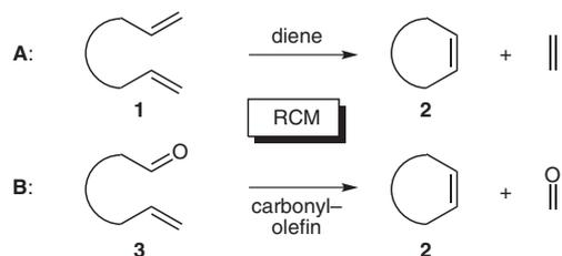
**Scheme 1** Ring-closing metathesis (RCM) starting either from a diolefin (diene metathesis; **A**) or from an unsaturated carbonyl compound (carbonyl–olefin metathesis; **B**)
