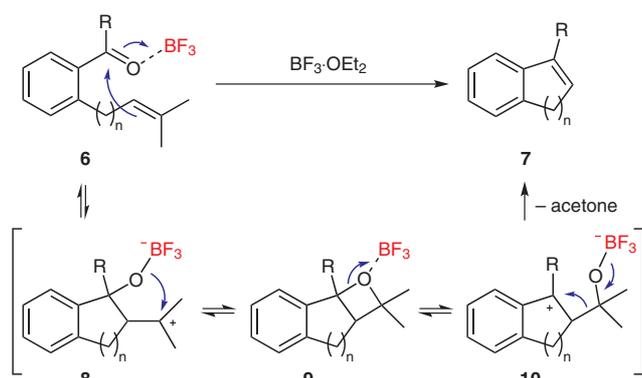
**Scheme 3** Proposed mechanism for the BF<sub>3</sub>-promoted metathesis cyclization of substrates of type **6**
