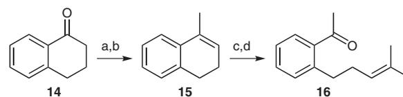
**Scheme 5** Synthesis of substrate **16**. Reagents and conditions: (a) MeMgI, EtO<sub>2</sub>, r.t., 1 h; (b) HCl (3 N), r.t., 1 h, 98% over 2 steps; (c) O<sub>3</sub>, MeOH, -78 °C, 4 h, then Me<sub>2</sub>S, r.t., 24 h, 35%; (d) *n*-BuLi, *i*-PrPPh<sub>3</sub>I, THF, -78 °C, 2 h, then r.t., 16 h, 30%.
