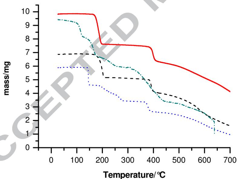
**Fig 4** TG records for the Ni(II)-Co(II) complexes: **I** – dashed, **II** – solid, **III** – dotted, **IV** – dot dashed.
