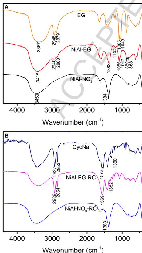
**Fig. 2.** FT-IR spectra of (A) NiAl-NO<sub>3</sub>, NiAl-EG and EG; (B) NiAl-NO<sub>3</sub>-RC and NiAl-EG-RC
