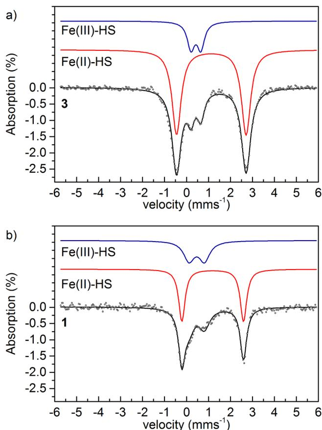
**Fig. 2.** Mössbauer spectra of a) **3** and b) **1** taken at 78 K. The black solid line is the sum of the subspectra originating from high-spin Fe(II) (middle) and high-spin Fe(III) (top). The parameters used for analysis are displayed in Table S1.
