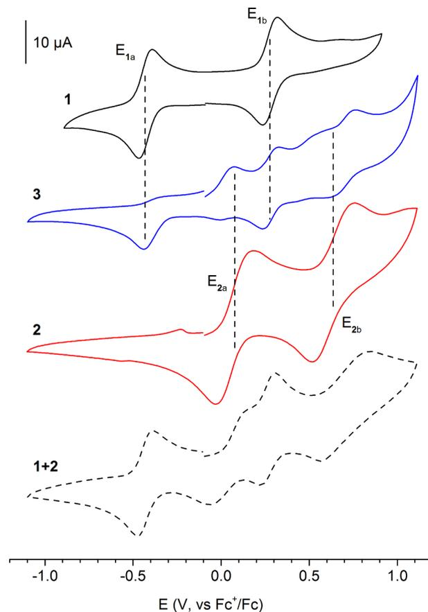
**Fig. 3.** Cyclic voltammetry of (top to bottom) **1**, **3**, **2**, and a 1:1 mixture of **1** and **2** (dashed) in  $\text{CH}_3\text{CN}$  with 0.1 M TBA(ClO<sub>4</sub>) (scan rate 100 mV/s). The half wave potentials for Fe(III)-Fe(II)/Fe(II)-Fe(II) ( $E_{1a}$ ) and Fe(III)-Fe(III)/Fe(III)-Fe(II) ( $E_{1b}$ ) from **1** and Mn(III)-Mn(II)/Mn(II)-Mn(II) ( $E_{2a}$ ) and Mn(III)-Mn(III)/Mn(III)-Mn(II) ( $E_{2b}$ ) from **2** are indicated by dashed vertical lines.
