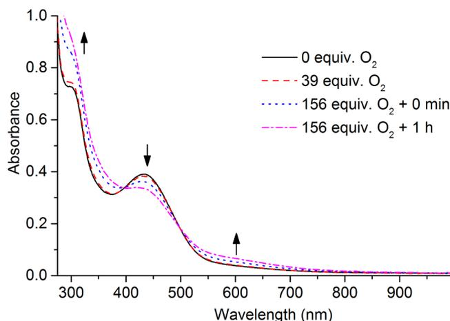
Fig. 5. Complex **1** ( $0.15$  mM) in  $CH_3CN$  (solid line) and with added equivalents of  $O_{2(g)}$  (coloured traces). The solubility of  $O_2$  in pure acetonitrile at  $20^\circ C$  is  $2.4$ – $2.6$  mM [49–50].
