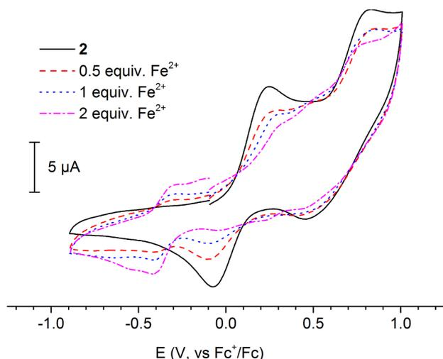
Fig. 4. Cyclic voltammetry in  $CH_3CN$  ( $0.1$  M  $TBA(ClO_4)$  as electrolyte) following the titration of **2** ( $1$  mM) with  $Fe(CH_3CN)_6(PF_6)_2$ .
