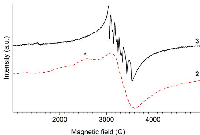
**Fig. 1.** EPR spectra of **3** (top) and **2** (bottom, dashed) in  $\text{CH}_3\text{CN}$  at 5 K. The characteristic peak from **2** at  $g \sim 2.6$  is marked with an asterisk (\*). Microwave power, 20  $\mu\text{W}$ .
