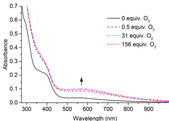
Fig. 6. Complex **3** (0.15 mM) in CH<sub>3</sub>CN (solid line) and with added equivalents of O<sub>2(g)</sub> (coloured traces). The solubility of O<sub>2</sub> in pure acetonitrile at 20 °C is 2.4–2.6 mM [49–50].
