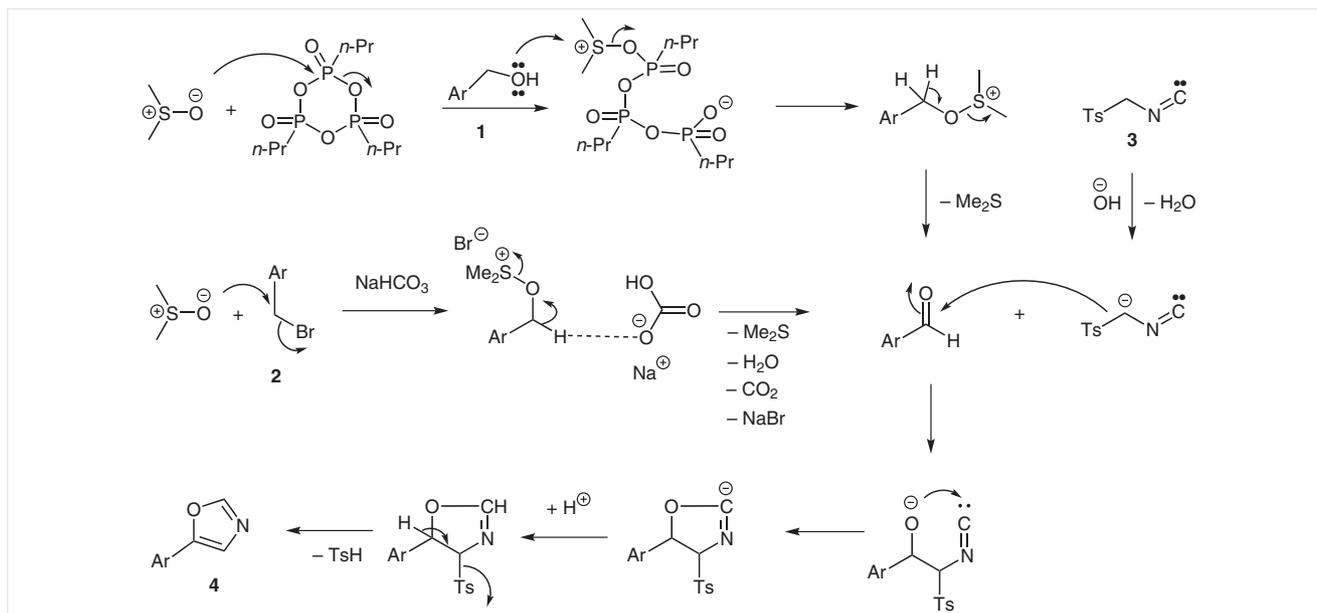
**Scheme 1** The plausible mechanism for the synthesis of 5-aryl oxazoles from benzyl alcohols and benzyl bromides.
