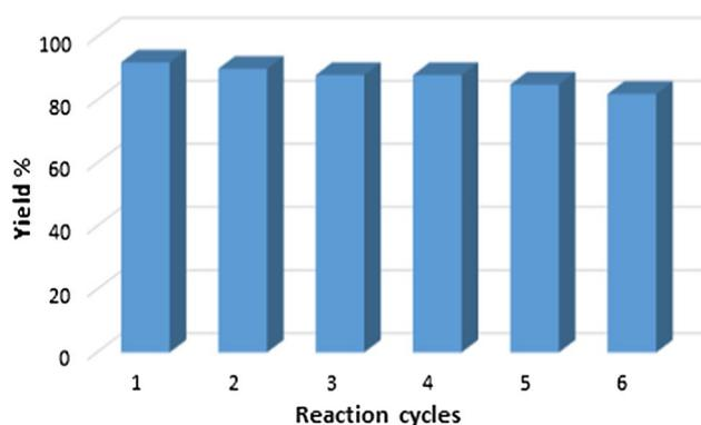
**Fig. 6** Recyclability of the NS-CSs catalyst in the Kabachnik–Fields reaction
