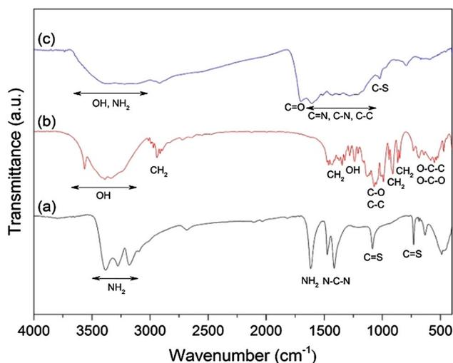
**Fig. 4** FTIR spectra of *a* thiourea *b* sucrose *c* NS-CSs
