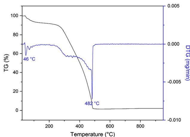
**Fig. 5** TGA and DTG curves of NS-CSs
