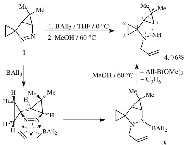
Scheme 1. Reaction of pyrazoline **1** with triallylborane.
