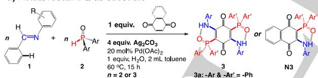
**Scheme 1.** Pd(II)-catalyzed C-C or C-P bond formation with 1,4-benzoquinone employed as co-catalyst (**1a**,<sup>11a</sup> **1b**<sup>21</sup>) or substrate in this work (**1d**).
