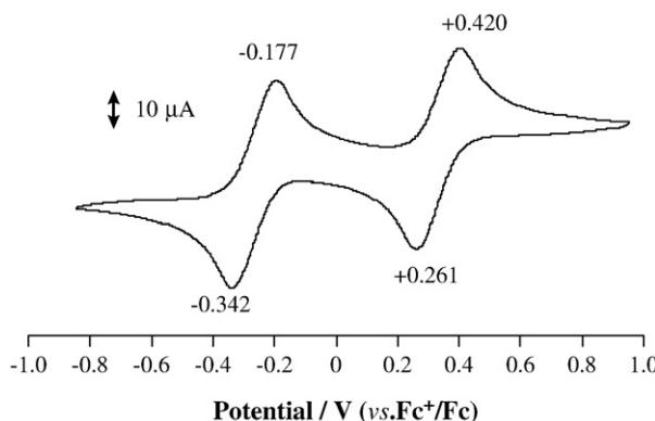
Fig. 4. Cyclic voltammogram of  $[Pt(L)(cod)]$  in  $\text{CH}_2\text{Cl}_2$ .
