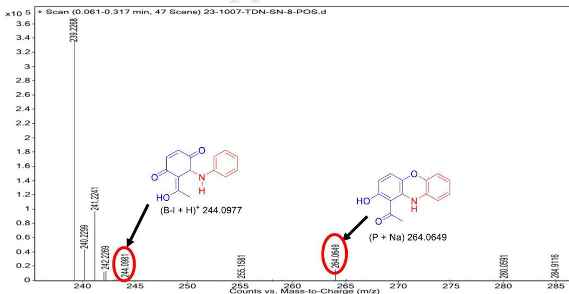
**Figure 2C.** ESI-MS of the reaction mixture, 5h after the addition of aniline to quinacetophenone. The signals due to  $[B-l + H]^+$  and  $[P + H]^+$  are encircled.
