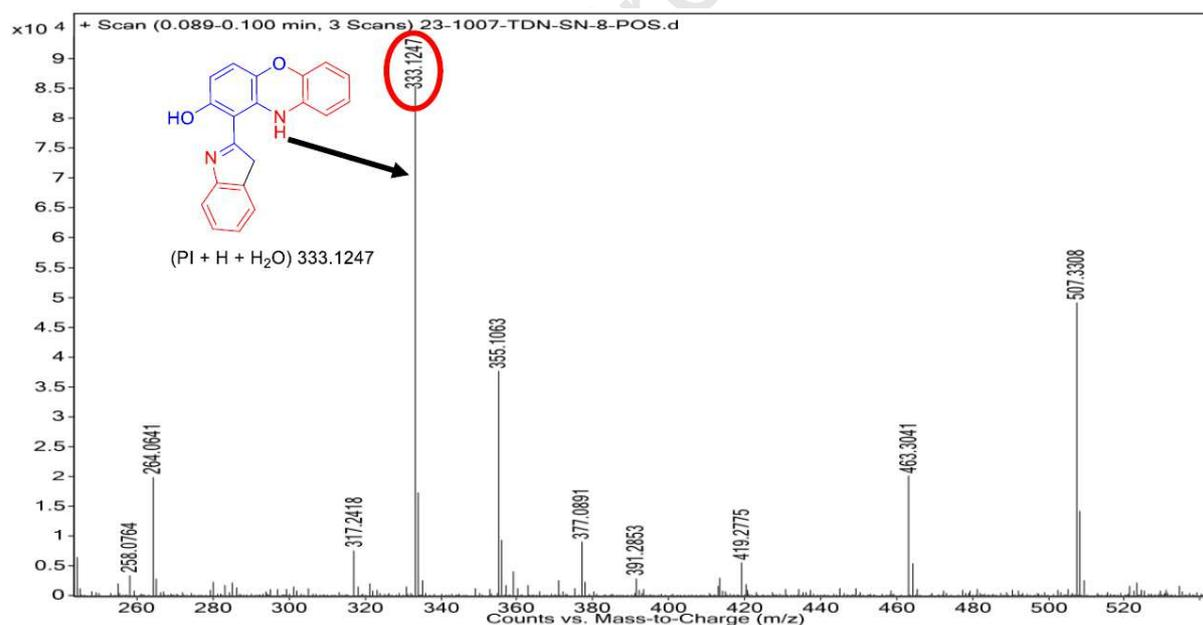
**Figure 2E.** ESI-MS of the reaction mixture 5h after the addition of aniline to quinacetophenone. The signals due to  $[PI+H_2O+H]^+$  are encircled.
