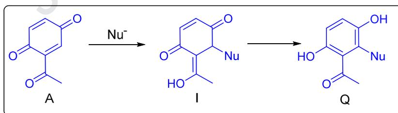
**Figure 1.** 2-acetyl 1,4- benzoquinone (**A**); Intermediate (**I**) and formation of 6-substituted quinacetophenone (**Q**) by rearomatization
