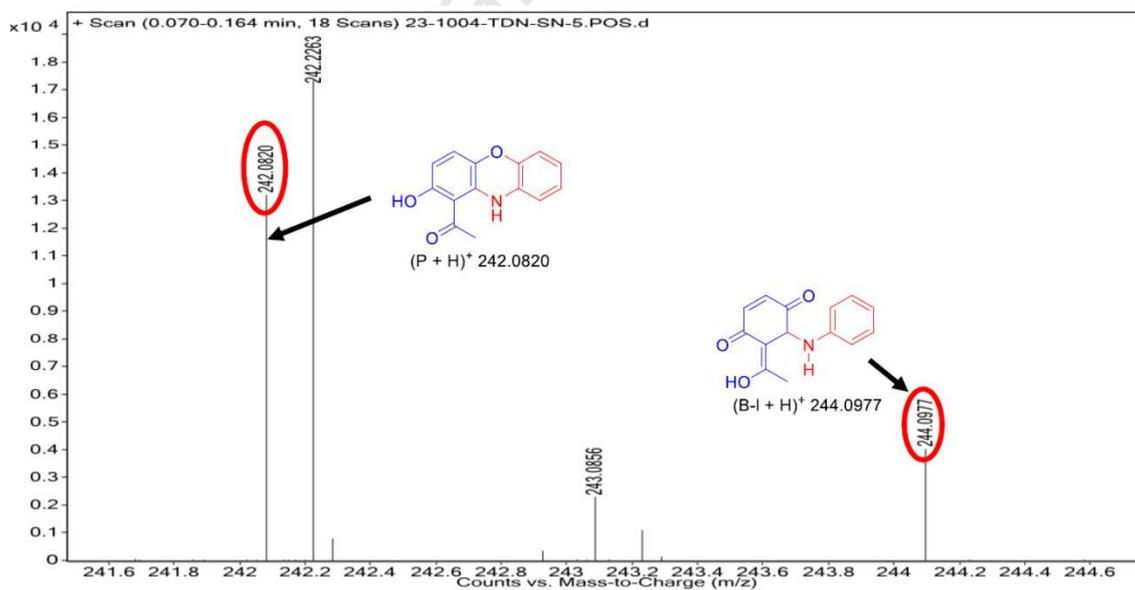
**Figure 1A.**ESI-MS of the reaction mixture, 1 min after the addition of aniline to quinacetophenone. The signals due to species  $[\mathbf{B-I} + \mathbf{H}]^+$   $[\mathbf{P} + \mathbf{H}]^+$  are encircled.
