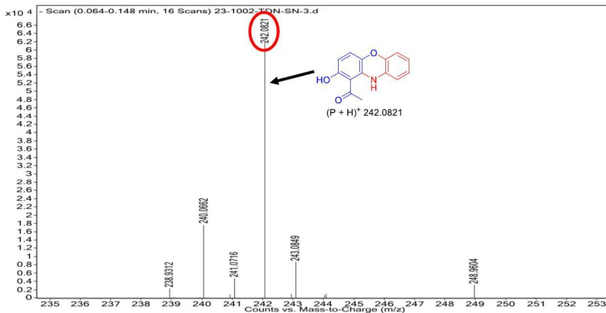
**Figure 2B.** ESI-MS of the reaction mixture, 1.5 h after the addition of aniline to quinacetophenone. The signals due to species  $[P + H]^+$  are encircled.
