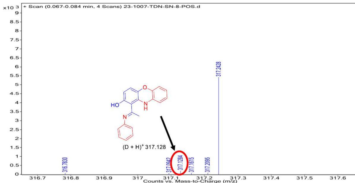
**Figure 2D.** ESI-MS of the reaction mixture, 5h after the addition of aniline to quinacetophenone. The signals due to  $[D+H]^+$  are encircled.
