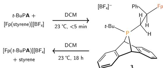
**Scheme 2.** Reaction of *t*-BuPA with  $[\text{Fp}(\text{styrene})][\text{BF}_4]$ .
