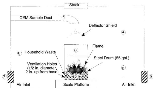
FIGURE 1. Burn hut diagram (numbers represent thermocouple locations).
