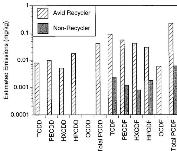
**FIGURE 3. Congener distribution of PCDDs/PCDFs. Results are averaged across duplicate run conditions with nondetects set to zero. Note that OCDD data are suspect due to the presence in hut blank samples and are not shown.**
