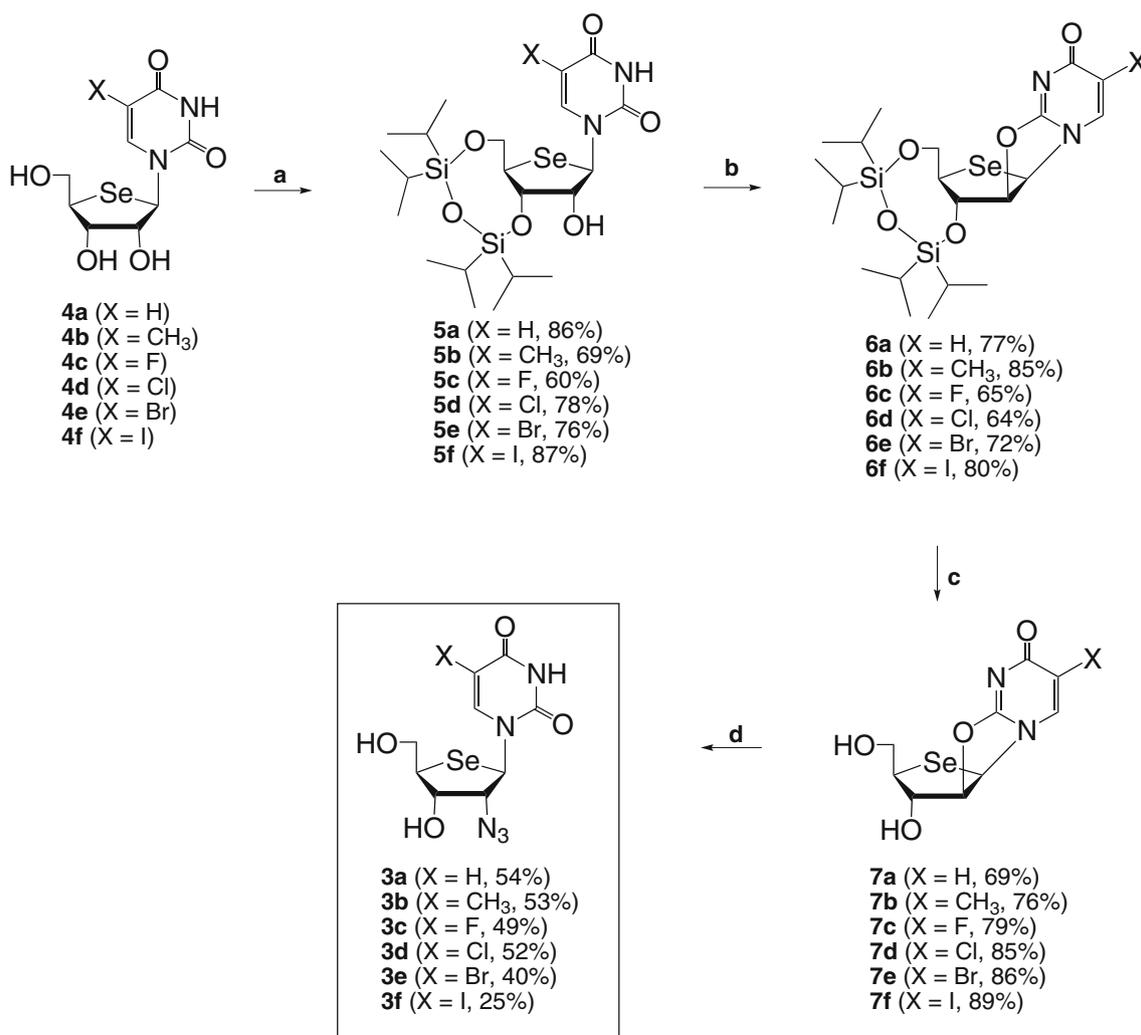
**Scheme 1** Reagents and conditions: (a) TIPSCl<sub>2</sub>, pyridine, rt, 3 h; (b) DAST, MC, -78 °C, 1 h or MsCl, then DBU; (c) 3HF-Et<sub>3</sub>N, THF, 0 °C, 1 h; (d) NaN<sub>3</sub>, DMF, 120 °C, overnight
